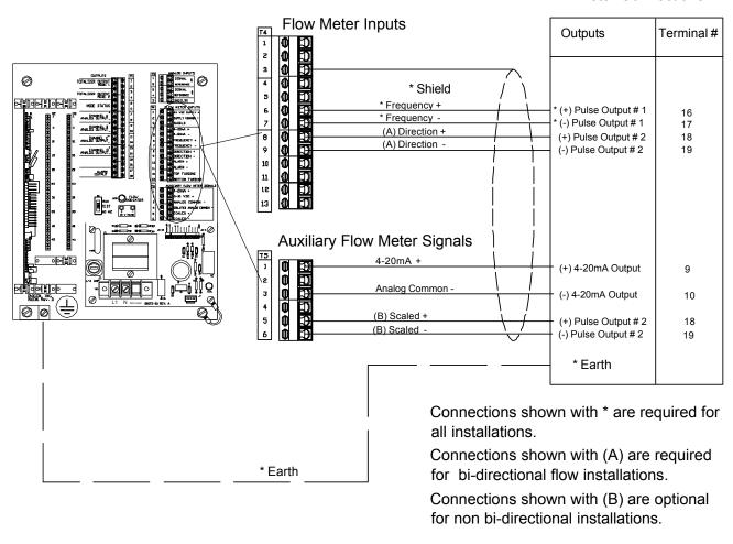
Note: The D-100 does not provide power to the F-3100 or F-3200 flow meter. Input power for the flow meter must be provided separately. See flow meter manual for detailed wiring instructions.
