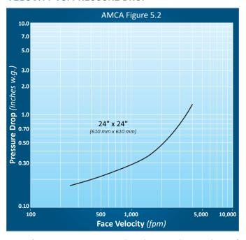
Air Performance testing was conducted in accordance with ANSI/AMCA Standard 500-D, Figure 5.2. Vertically mounted test damper is located at the end of 5 diameters of a duct run, exhausting into an open area. Both duct and test damper are downstream from air supply.
