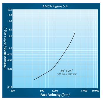
Air Performance testing was conducted in accordance with ANSI/AMCA Standard 500-D, Figure 5.4. Data are based on a vertically mounted damper.
