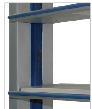
Appearance of damper seals after cycle testing
