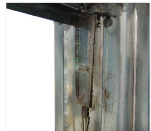
Appearance of damper seals after cycle testing
