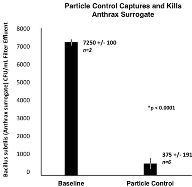
**Fig 3.** Particle control kills anthrax surrogate. The collector surface was loaded with >100 million viable *Bacillus subtilis* cells at a surface loading density >10<sup>7</sup> cells/cm<sup>2</sup>. Within 3 hours of exposure, particle control technology killed 95% of the anthrax surrogate *B subtilis* ( $P < .0001$ ). CFU, colony-forming units.
