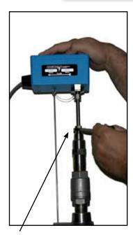
Step 1: Slowly loosen the position clamping nut while maintaining a firm grip on the enclosure to counteract the effect of pressure in the pipe.
